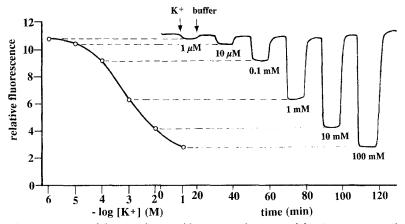
Fig. 5. Calibration graph and response curve of the potassium-sensitive pvc membrane containing 2a as proton carrier and TOP as plasticizer, at pH 7.38.
